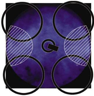
Fig. 20 Image of cylinder end view showing areas of preferential ignition sites as crosshatch
